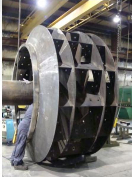
130" dia. Backward Inclined DWDI – Rotor Rebuild,
