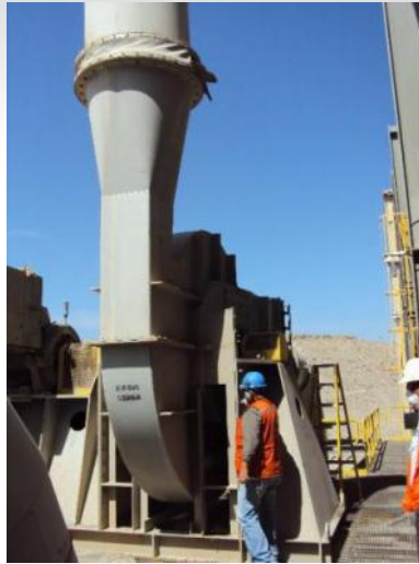
DRBS-2200 SR.25R DWDI, Radial Bladed Fan, Arr't 7
